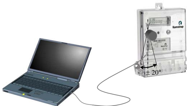
Figure 3: Hardware set-up for a laptop with METERTOOL and an optical head
