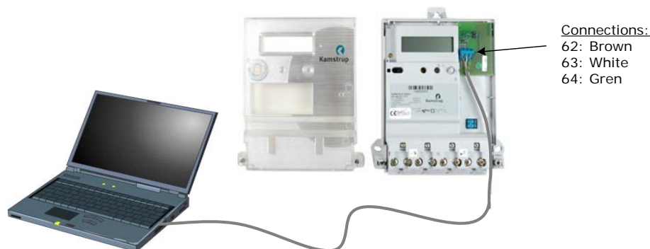
Figure 4: Hardware set-up for a laptop with METERTOOL and a data/pulse module
